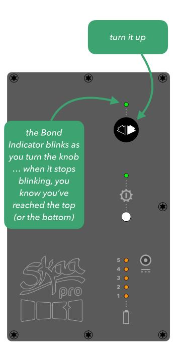
DFB is a proper SKAA receiver ... and as with every SKAA receiver, volume control is done at the last possible point in the signal chain; in this case, it happens inside DFB's amplifiers. SKAA sends your audio full scale (not scaled by the volume level) over the air. This is to ensure you always get the best possible Signal to Noise Ratio (SNR) regardless of the volume level
