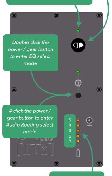
Use the LED stack to navigate through the EQ and Audio Routing Options
