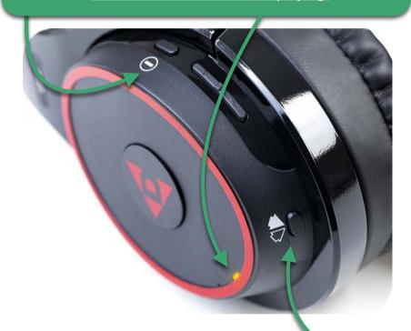
If the Bond Indicator stays dim Amber and you don't hear any audio, carry out a factory reset by quickly clicking the Bond Button 6 times. Your click speed should be similar to multi-clicking a computer mouse.
