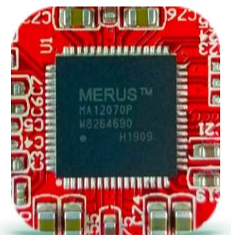
At the heart of Aquarius is its Merus™ amplifier - Infineon's most efficient audio amp. Merus boasts a stellar 92% efficiency, meaning that more of your battery's power is converted into sound and not into heat. More power savings means more hours of music giving Aquarius its 36+hour battery life at normal listening levels.
