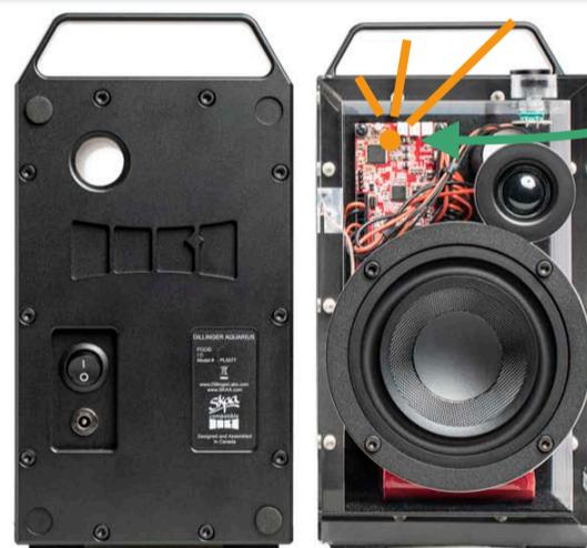
If the Bond Indicator stays dim Amber and there is no audio, Factory Reset by clicking the Bond Button 6 times. The Bond Indicator will flash Red if the reset is successful.
