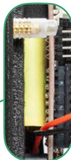
Film capacitors are an audio engineer's best friend! When an amplifier demands power, not all capacitors are capable of supplying an instantaneous flow of charge; this is where a film capacitor comes to the rescue. Next time you hear a kick drum in your Aquarius speakers, remember the film capacitor makes it happen with an extra punch.
